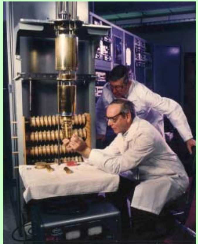
Figure 4: Bill Steele showing Dennis Ripley the fine detail of one of the adiabatic calorimeters. Note in the background the spools of fine wire needed to construct the temperature control portions of the equipment.
